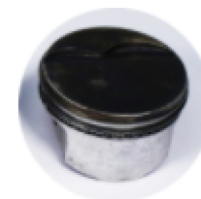
High carbon deposit on piston heads
