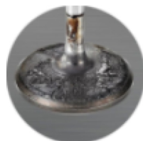
High carbon deposit on engine valves
