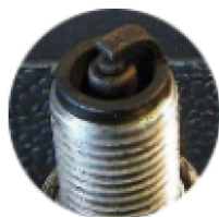
High carbon deposit on spark plugs
