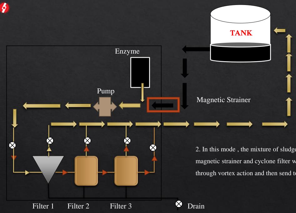
2. In this mode, the mixture of sludge and enzyme are sent via magnetic strainer and cyclone filter where impurities are separated through vortex action and then send to the tank.
