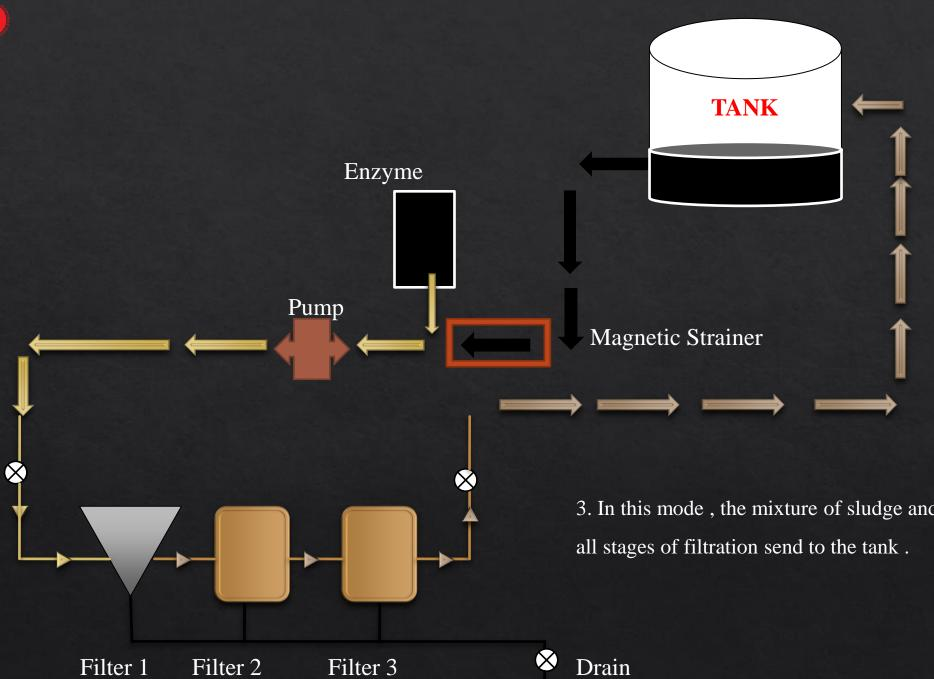
3. In this mode, the mixture of sludge and enzyme are passed through
